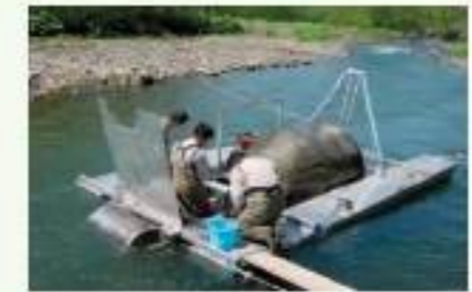
Survey on the fry flowing-down by a screw trap.
